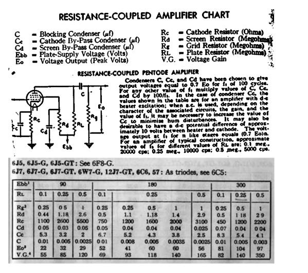
Modified to triode stage with relatively low stage gain ~15, but total amp gain was too low, so reverted to pentode mode with 680R cathode, 100k anode load, and 470k screen.
